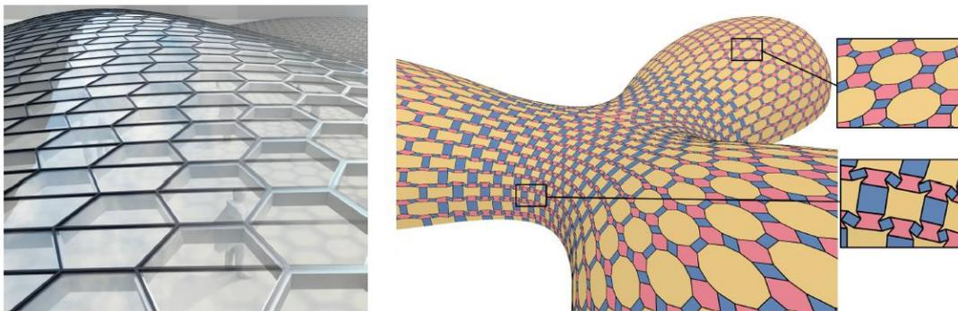
**Figure 1:** Polyhedral patterns. Left: A quad mesh needs not look like a curved regular grid. Right: In positively curved areas, the pattern appears like the corresponding semi-regular pattern in the plane, but in negatively curved areas it changes significantly.
