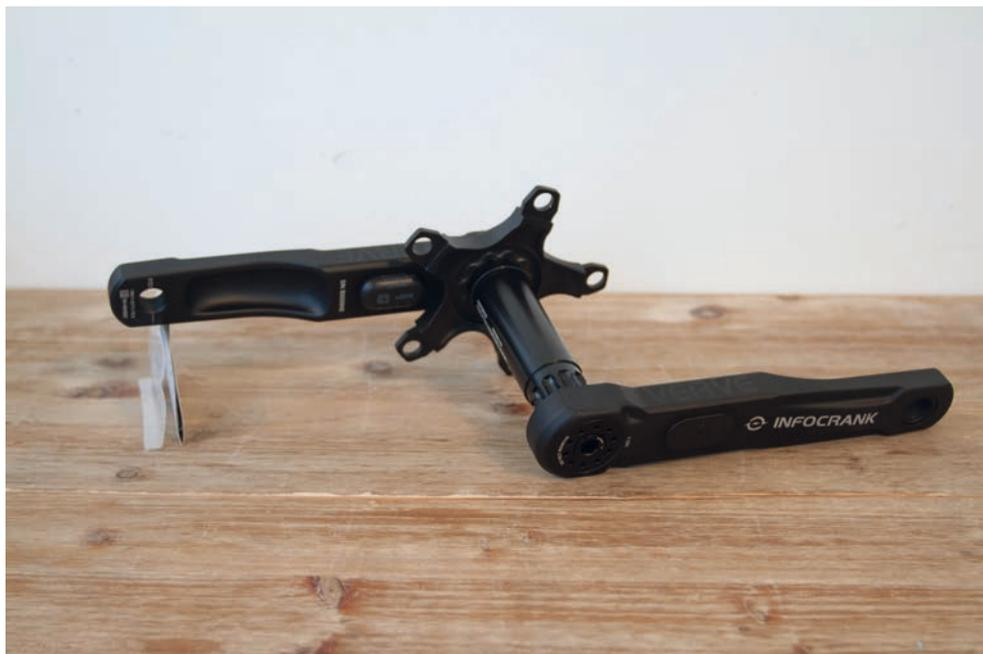
Abb. 24: Kurbelarm-Powermeter Infocrank BCD
