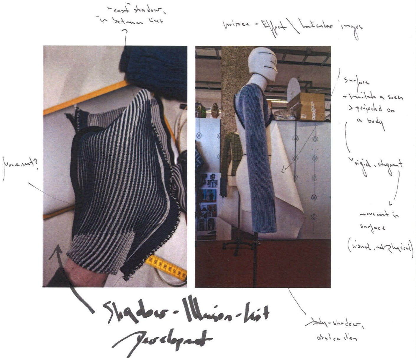
● Shadow-Illusion Knit, Developed with Nina Dorfer on the Stoll CMS 822, 10 Gauge
