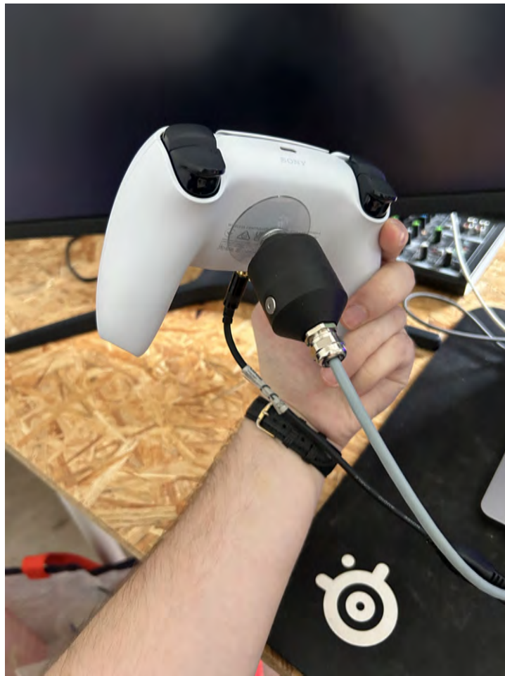
Figure 2.33: Recording setup of Playstation 5 gamepad DualSense, contact microphone Lom Geofon mounted with suction piece.
