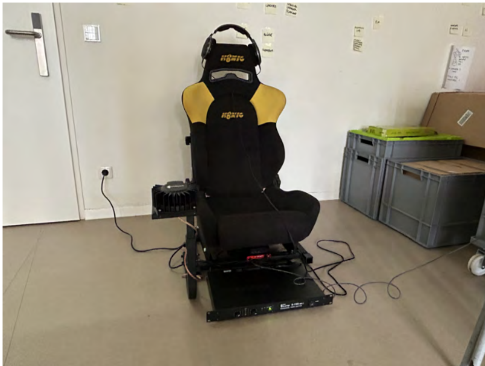
Figure 4.6: Fully assembled playback system with seat of Embracing Sphere installation. Power amplifiers for VCA's are visible in front of the seat.
