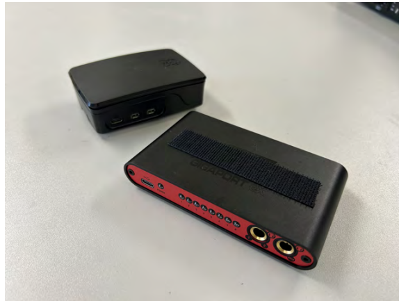
Figure 4.2: Processing and digital audio converter units of the Embracing Sphere installation. Raspberry Pi 5 and ESI GigaPort EX.
