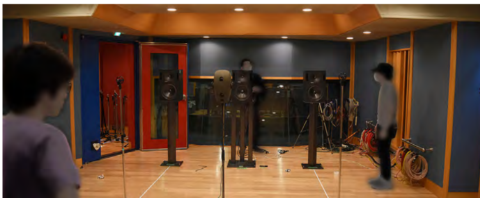
Figure 2.10: A visual of a RIR capturing session in a studio using sine sweep method. Retrieved from Audioease website https://www.audioease.com/altiverb/browse.php
