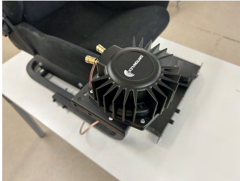
Figure 4.4: First bass shaker positioned on the right hand.
