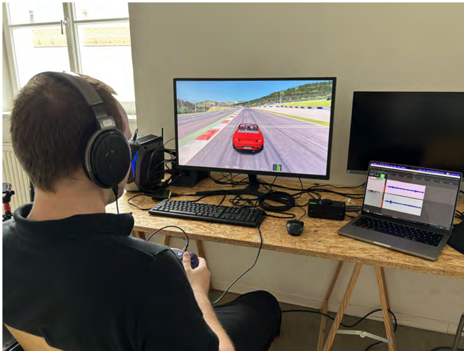
Figure 4.9: A picture from a simulation rumble signal sampling session. Assetto Corsa (a vehicle simulation game, developed by Kunos in 2013) and sim-hub (an add-on tool for telemetry logging and generating rumble signal with telemetry data accessed from simulation) were used for vehicle simulation, recorded through a sound card.
