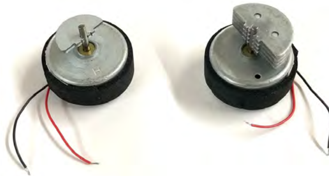
Figure 1.7: Vibration motors of Dualshock 2.
