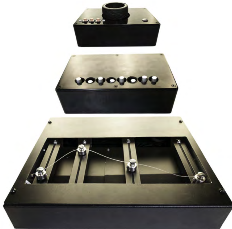
Figure 3.9.5: Tangible interfaces - tangible wheel , tangible pins and tangible string (top to bottom).
