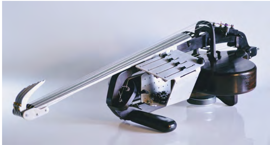
Figure 1.5.3: Halldorophone by Halldór Úlfarsson at NIME 2018: “a new electroacoustic string instrument which makes use of positive feedback as a key element in generating its sound” [Úlfarsson 2018]
