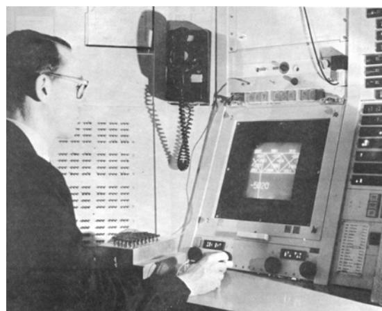
Figure 2.2.2: Ivan Sutherland’s Sketchpad 1963 was the first graphical computer interface. On the display a drawing can be seen, as well as the light-pen in the hand that enables drawing lines on the screen.
