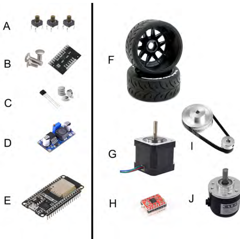
Figure 3.5.8: Tangible Wheel - components. (A) tact switch push buttons (B) capacitive touch board and steel screws (C) neodymium magnets and hall sensor (D) DC-DC step down converter (E) ESP 32 micro-controller (F) race car rubber wheel (G) stepper motor (H) motor control board (I) aluminium gear wheels and rubber belt (J) rotary encoder.
