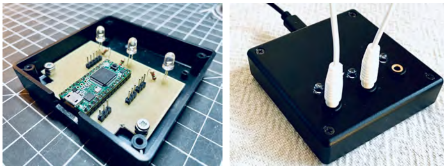
Figure 3.8.3: Development of MIDI interface using a micro-controller. Figure 3.8.4: MIDI interface with two serial connections.
