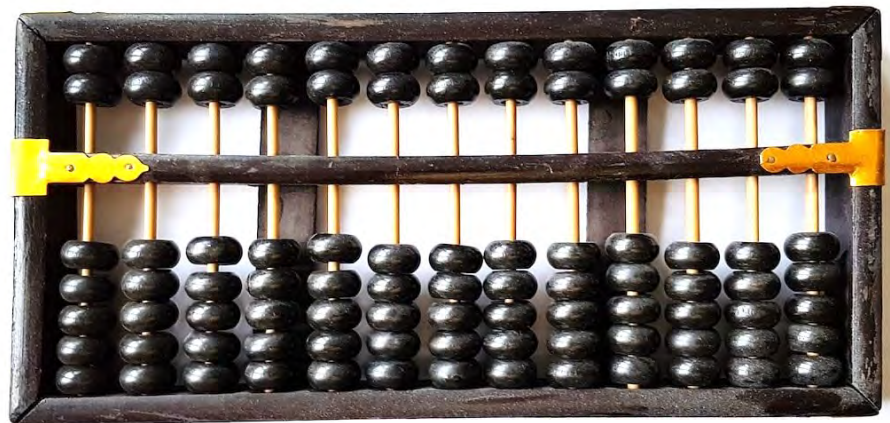
Figure 2.4.1: Chinese Suan Pan Abacus (around 190 CE). Calculations like addition, subtraction, multiplication and division can be realized by following a bi-quinary coded decimal encoding scheme.
