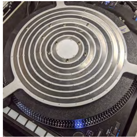
(b) Tamphall8r static part with 8 rotatable concentric rings
