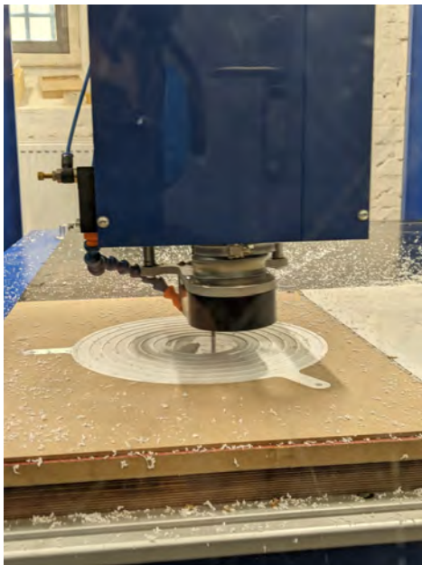
Figure 3.6: Photo of the Tamphall8r rings during CNC milling
