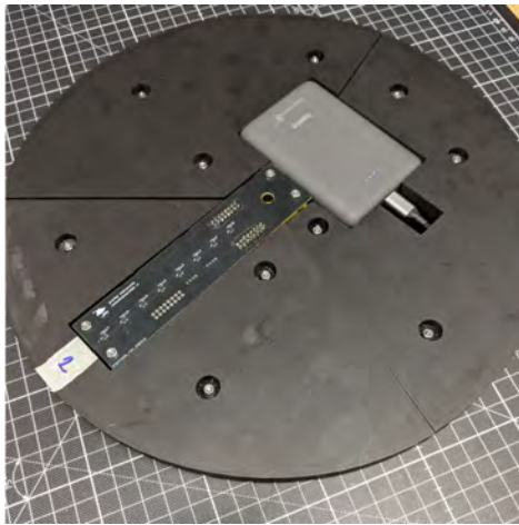
(a) Tamphall8r rotating part with 8 Hall effect sensors
