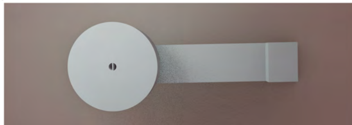
Figure 4.32: Lever design for a potentiometer
